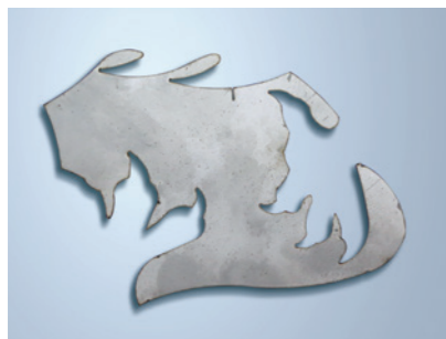
普通切割方式，转角挂渣 Standard Cutting Dross around the Corner
