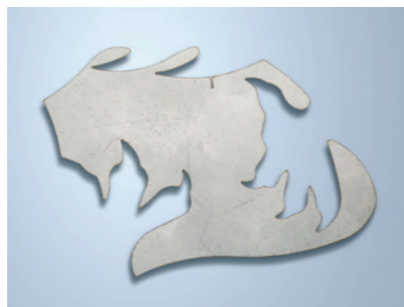
GC系统切割方式，转角无挂渣 Cutting with GC Controller Without Dross around the Corner
